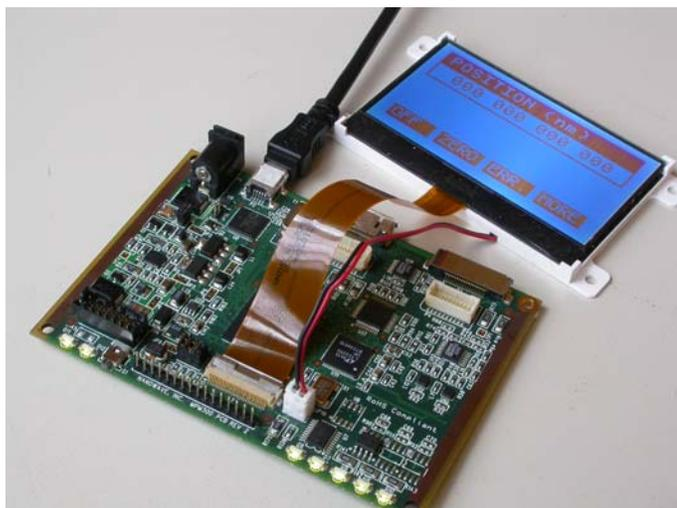
**Figure 1. USB Powered MPM300/OEM with LCD Display**
